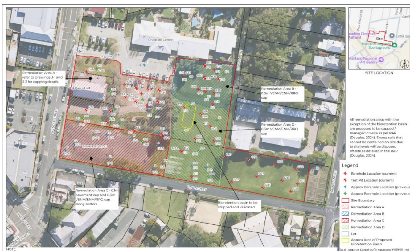
Figure 2 – Site boundary, remediation area, proposed capping & depth of impacted fill
